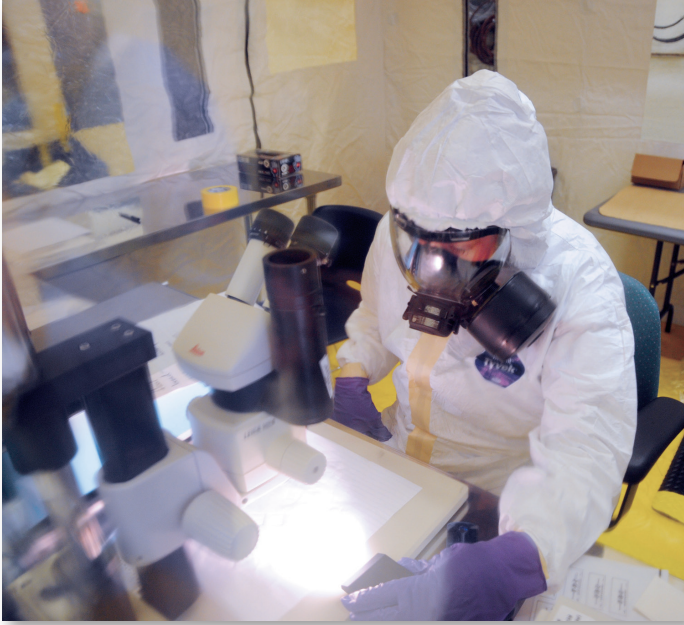
A Trace Evidence examiner uses oblique light to aid in finding hairs, fibers, or similar small material that might be deposited on an item of evidence from a radiological crime scene
