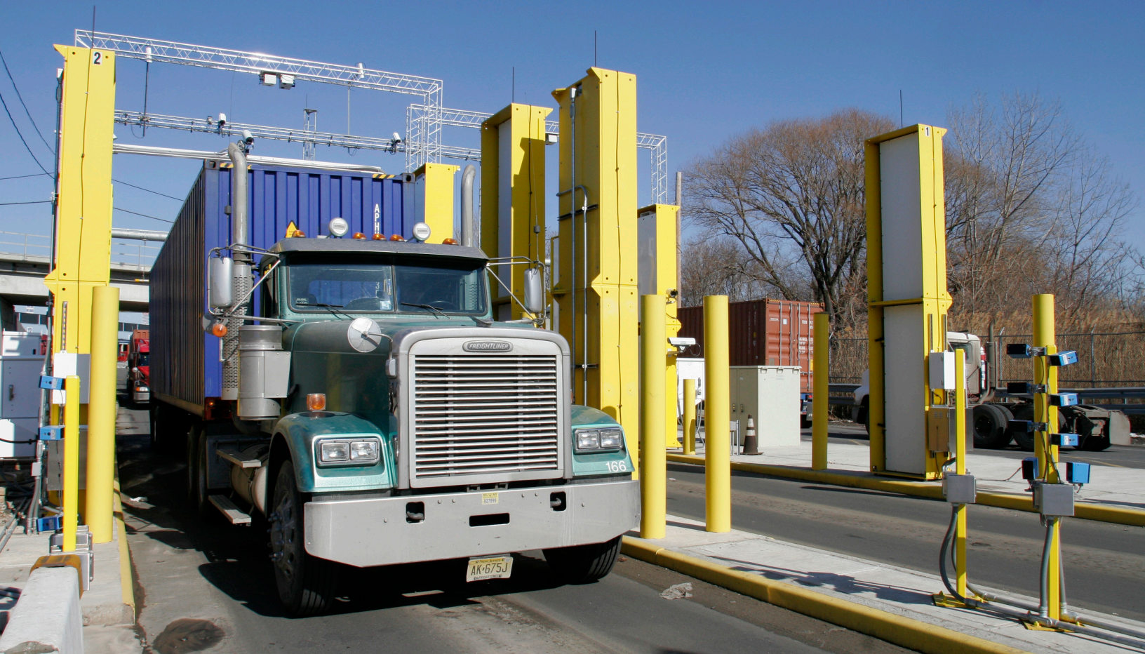
A truck passes through a radiation portal monitor. Such devices are used to guard borders and nuclear facilities.
